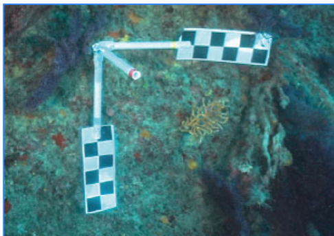
Fig.1. Example of a ground control point. The dimension of this GCP was 22 cm _ 22 cm _ 22 cm. The chessboard extension was 21 cm long by 8 cm wide, but size can be different, it is a reference point useful to correctly reconstruct the surveyed area (Palma et al., 2018).
